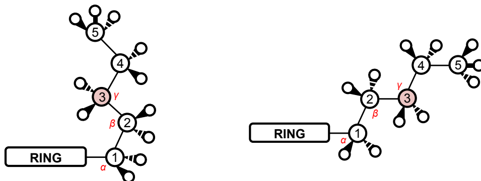
Figure 1-11. Illustrations of gauche (left) and trans (right) primary conformation.
