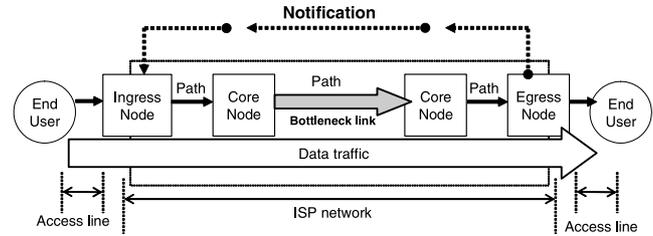
Fig. 2 Notification with one-way feedback control.
