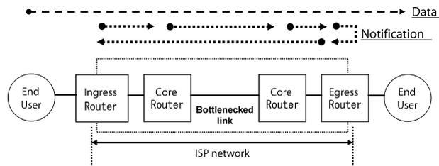
Fig. 1 Notification in roundtrip feedback control.
