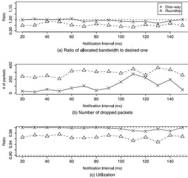
**Fig. 10** Effect of NI. (MI = 50 ms for one-way feedback control, MI = 100 ms for round-trip one)
