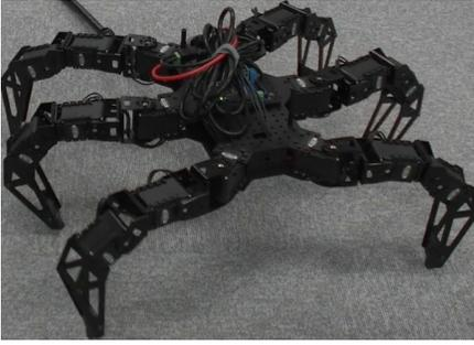
Fig. 7. PhantomX hexapod developed by Trossen Robotics. Each leg is controlled by inverse kinematics toward its reference given as an oscillator’s phase.
