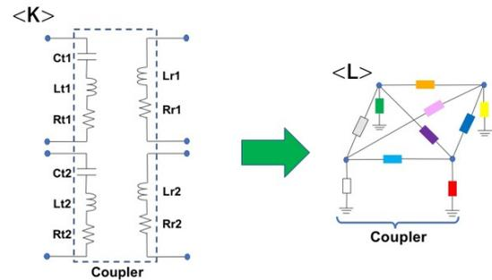
Fig. 5 Equivalent circuit of coupler including resistance
