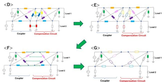
Fig. 2 Flow of canceling out reactance in the coupler
