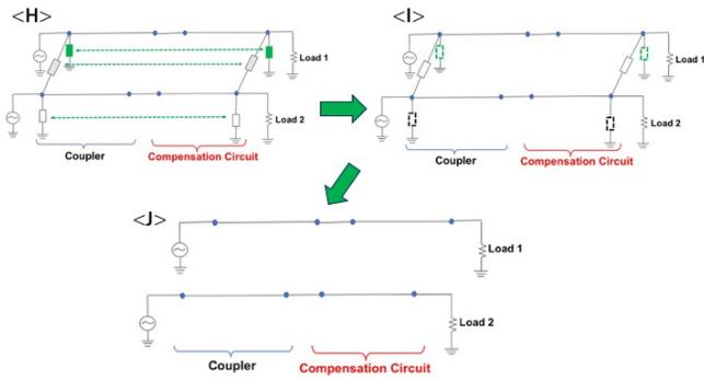
Fig. 3 Flow of canceling out reactance in the coupler
