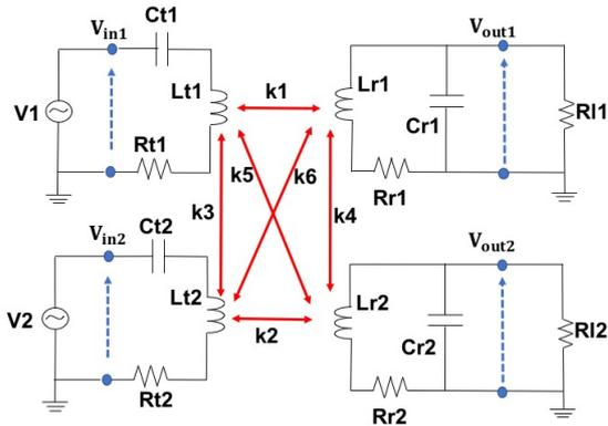
Fig. 6 Simulation model of SP method
