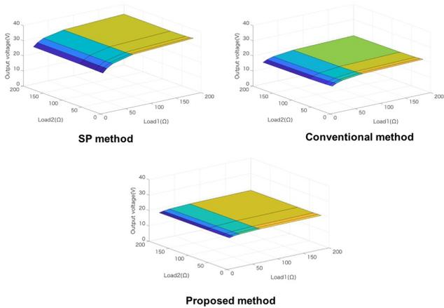
Fig. 9 Comparison of output voltage on load 1
