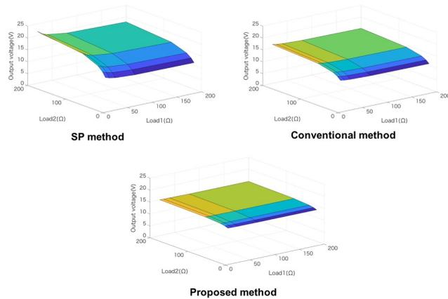
Fig. 10 Comparison of output voltage on load 2
