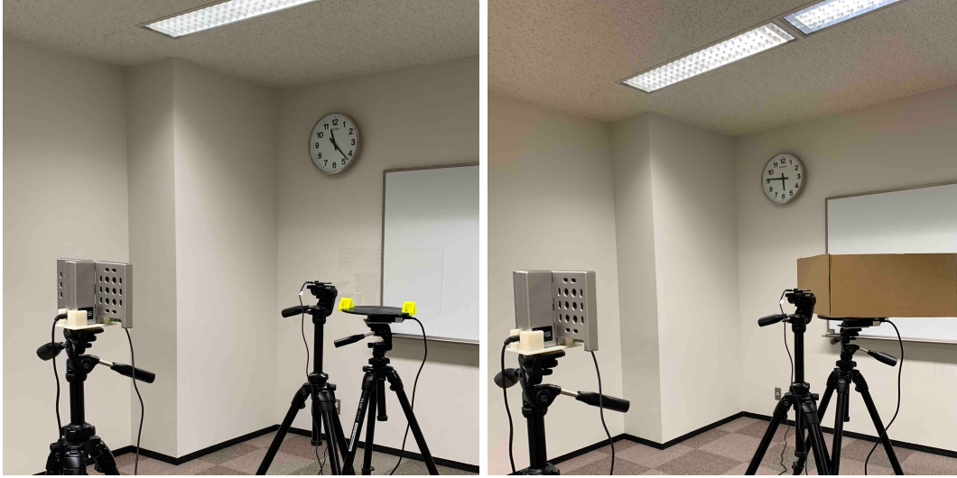
(a) Material is glass, Size is 200\text{mm} \times 400\text{mm} (b) Multiple plate (Material is cardboard, Size is 200\text{mm} \times 400\text{mm} \times 2\text{plate} )
