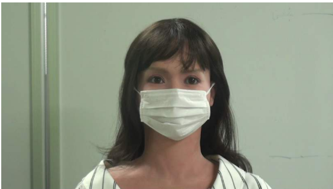
Fig. 2.15: Mask for hiding mouth movement
