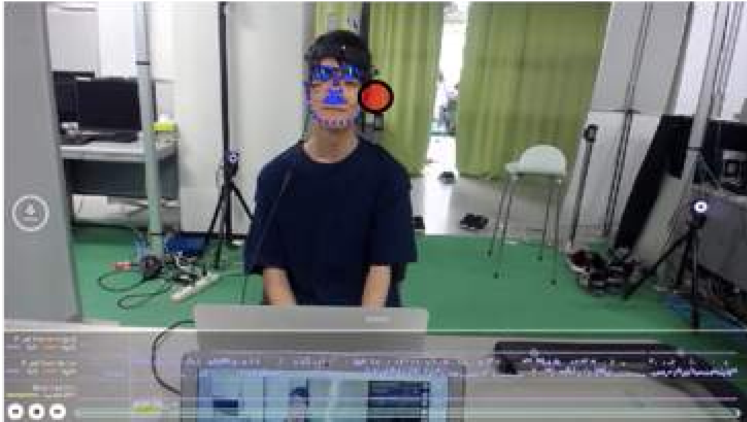
Fig. 2.4: A gaze point and face detection area in the automatic eye contact detection method
