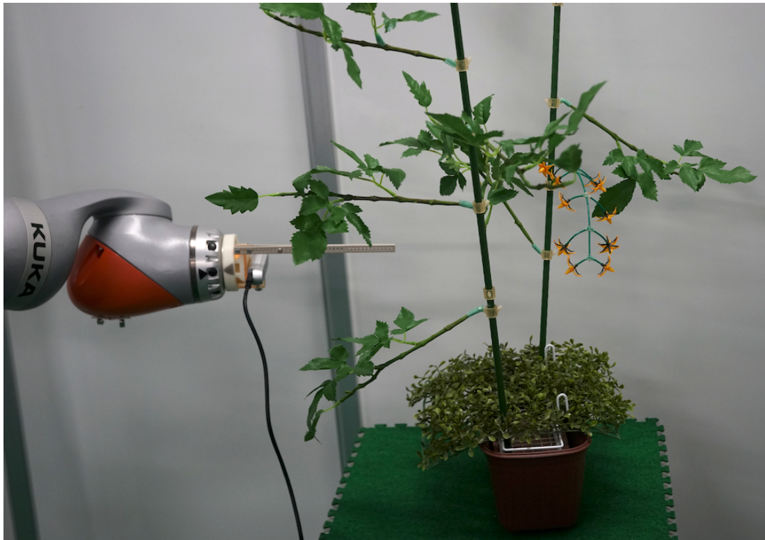
Fig. 35 Experiment for pollination of an artificial flower by the robot.
