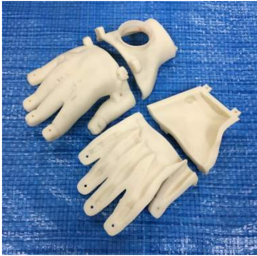
(a) The mold for fixing the bones
