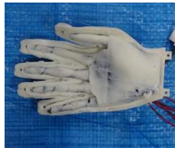
(f) Remove the mold of palm side
