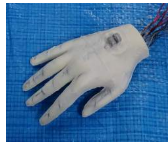
(h) Apply baby powder to the surface
