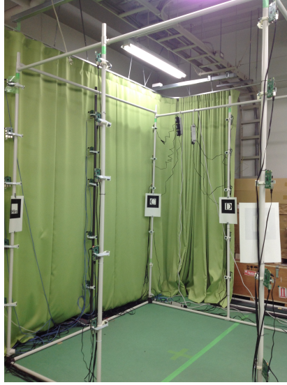
Figure 3.1: First version of the avatar acquisition system based on design from pi3dscan.
