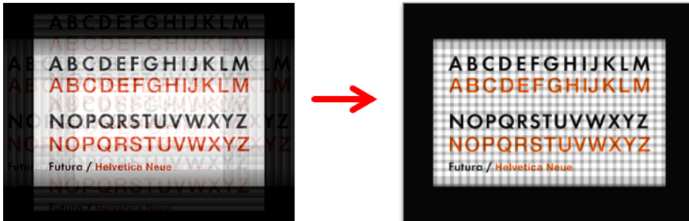
Figure 3.1.6: Retina image after removing ghost images
