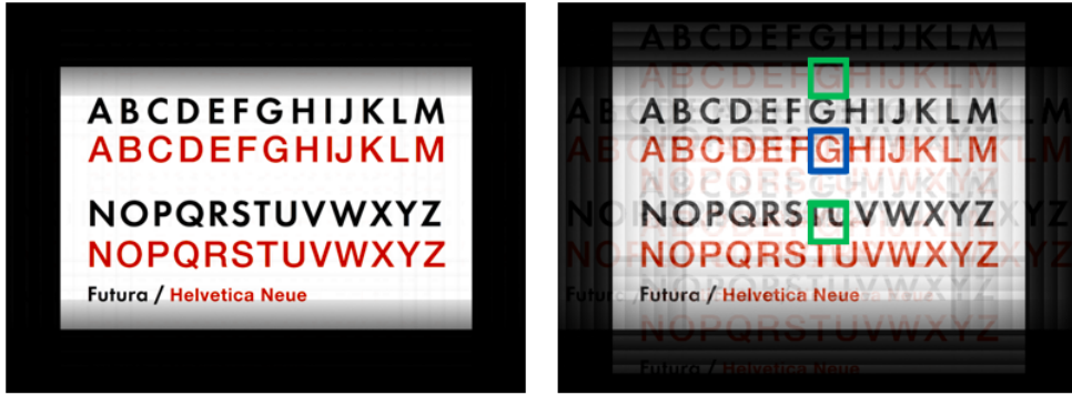
Figure 1.2.9: Normal case and ghost image case
