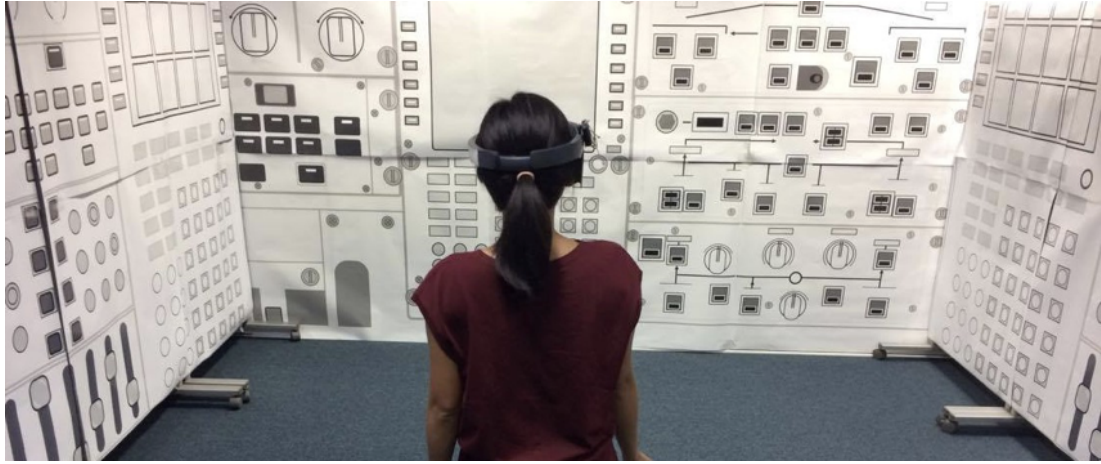
Figure 3.3: View of the control room with paper printouts on walls in the AR condition
