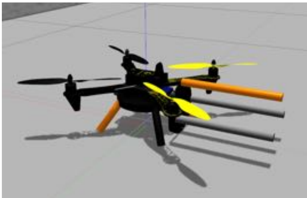
Fig. 4.5 Multi-Copter and End-effector
