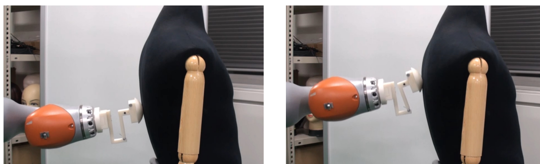
Fig. 4.4 Stroke motion with the cushioning mechanism
