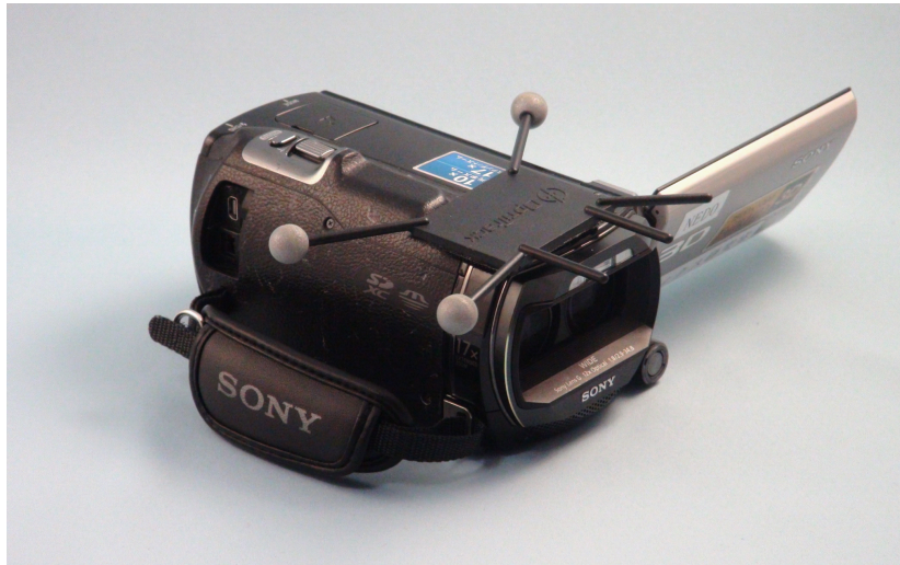
Fig. 3.3 A camera as a gaze direction object with reflective markers
