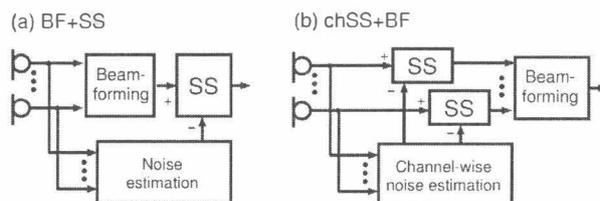
Fig. 1. (a) Block diagram of spectral subtraction after beamforming (BF+SS), and (b) channelwise SS before beamforming (chSS+BF).
