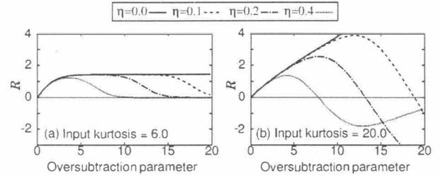
Fig. 5. Theoretical kurtosis ratio between chSS+BF and BF+SS for various oversubtraction parameters.
