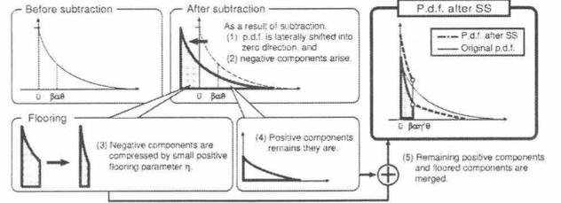
Fig. 2. Deformation of original p.d.f. of power-domain signal via SS.
