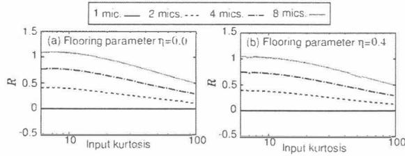
Fig. 4. Theoretical kurtosis ratio between chSS+BF and BF+SS for various values of input kurtosis.
