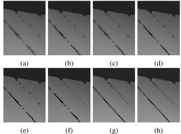
Fig. 1: Visual comparison among standard methods and curvelet domain regularization. (a) Markov Random Field (Kernel), (b) Markov Random Filed (2nd order smoothness), (c) Anisotropic Diffusion, (d) Bilateral Filter, (e) Noise Aware Filter, (f) Weight Mode Filter, (g) Curvelet Regularization, and (h) ground truth
