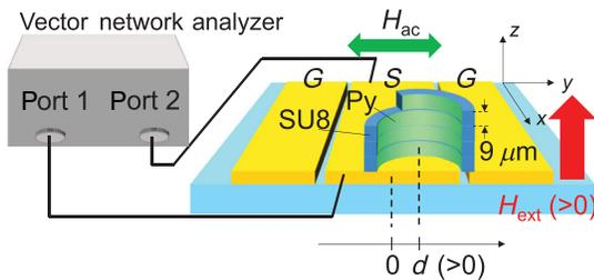
FIG. 1. Cross-section illustration of the CPW and the Py chiral metamolecule. The width of the center signal line (*S*) is  $82\ \mu\text{m}$  and the gap between the signal and ground (*G*) lines is  $9\ \mu\text{m}$ . The position of the metamolecule on the signal line is defined by the distance *d* between the signal-line center and the chiral axis.
