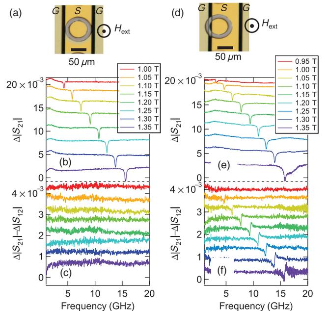
FIG. 4. Optical microscope images of Py rings with (a)  $d = 0 \mu\text{m}$  and (d)  $d = -20 \mu\text{m}$ . Signal lines of the CPW are highlighted in yellow. (b) and (e) are, respectively,  $\Delta|S_{21}|$  spectra of Py rings with  $d = 0 \mu\text{m}$  and  $d = -20 \mu\text{m}$  at various  $\mu_0 H_{\text{ext}}$  values. (c),(f) Corresponding directional differential spectra  $\Delta|S_{21}| - \Delta|S_{12}|$ .
