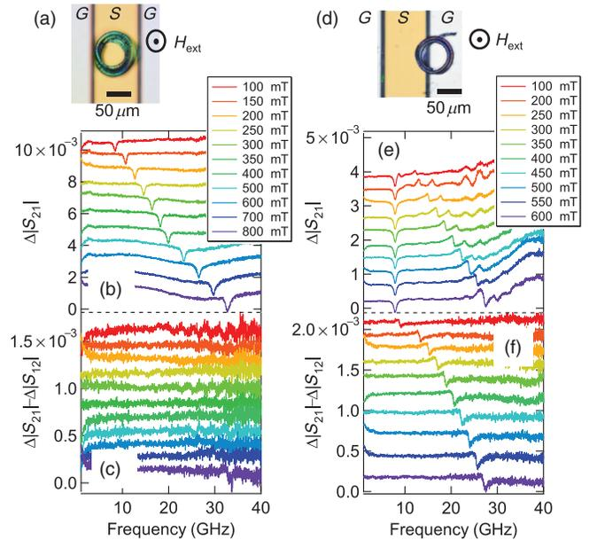
FIG. 2. Optical microscope images of a Py chiral metamolecule with (a)  $d = 0\ \mu\text{m}$  and (d)  $d = 60\ \mu\text{m}$ . Signal lines of CPW are highlighted in yellow. (b),(e) Corresponding microwave transmission spectra  $\Delta|S_{21}|$  at various external magnetic fields ( $\mu_0 H_{\text{ext}}$ ). (c) and (f) are the corresponding directional differential spectra  $\Delta|S_{21}| - \Delta|S_{12}|$ . (a) and (b) are reproduced from Ref. [8].
